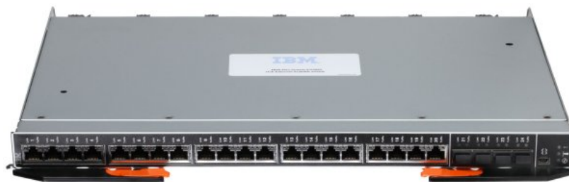
Figure 11: Chassis switch module
