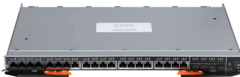
Figure 11: Chassis switch module
