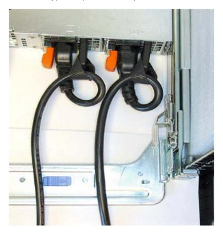
Figure 23: Proper PSU Cabling
