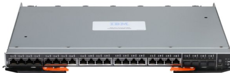
Figure 4: Chassis switch module
