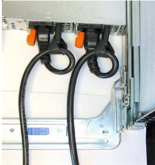
Figure 10. Proper PSU Cabling
