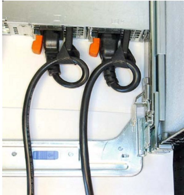
Figure 10. Proper PSU Cabling
